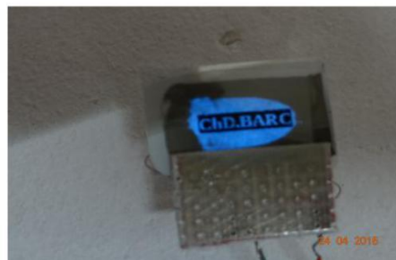
EL device of Zinc Sulphide doped with Copper ions
