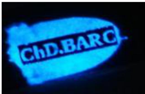
EL device of Zinc Sulphide doped with Copper ions
